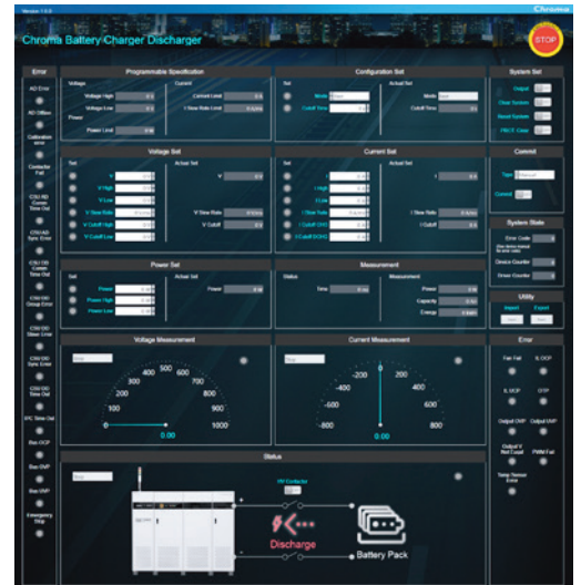
Battery Charge & Discharge interface
